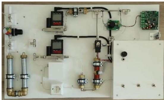
Figure 2: Picture of the assembled setup. The current version is intended for permeation tubes, but saturation chambers have been the most practical source in early testing.
