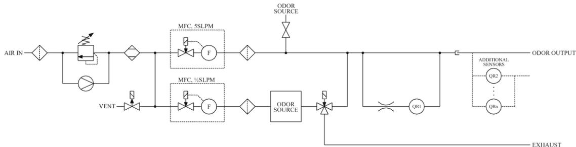
Figure 1: Block diagram of the OD and sensors.
